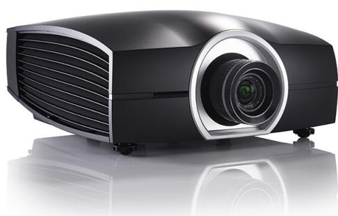
Producing a noise level of just 35dB, the Barco laser phosphor projectors are the quietest laser phosphor projectors currently available.\* Designed for fixed installation, the compact and lightweight PGWU-62L-K projector features WUXGA resolution (1,920 x 1,200). Its laser phosphor light source offers long lifetime, low maintenance (no lamps, no filters) and great color performance.
