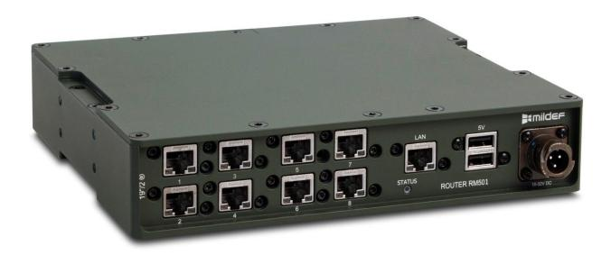
This rugged 19"/2® VoIP Gateway RM501 can offer a high port density in the smallest of space on one 19"/2 height unit. Up to up 8 analogue telephones and fax devices can be integrated into the VoIP network. It supports the fax-over-IP protocol T.38 especially for fax communication, which is the best way to enable stable fax transmission over IP routes.
