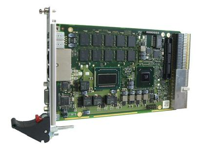
The F21P can be extended by different side cards. Additional functions include a digital video interface for flat panel connection via DVI (multimedia), a variety of different UARTs or another four USBs, SATA for hard disk connection and HD audio.
