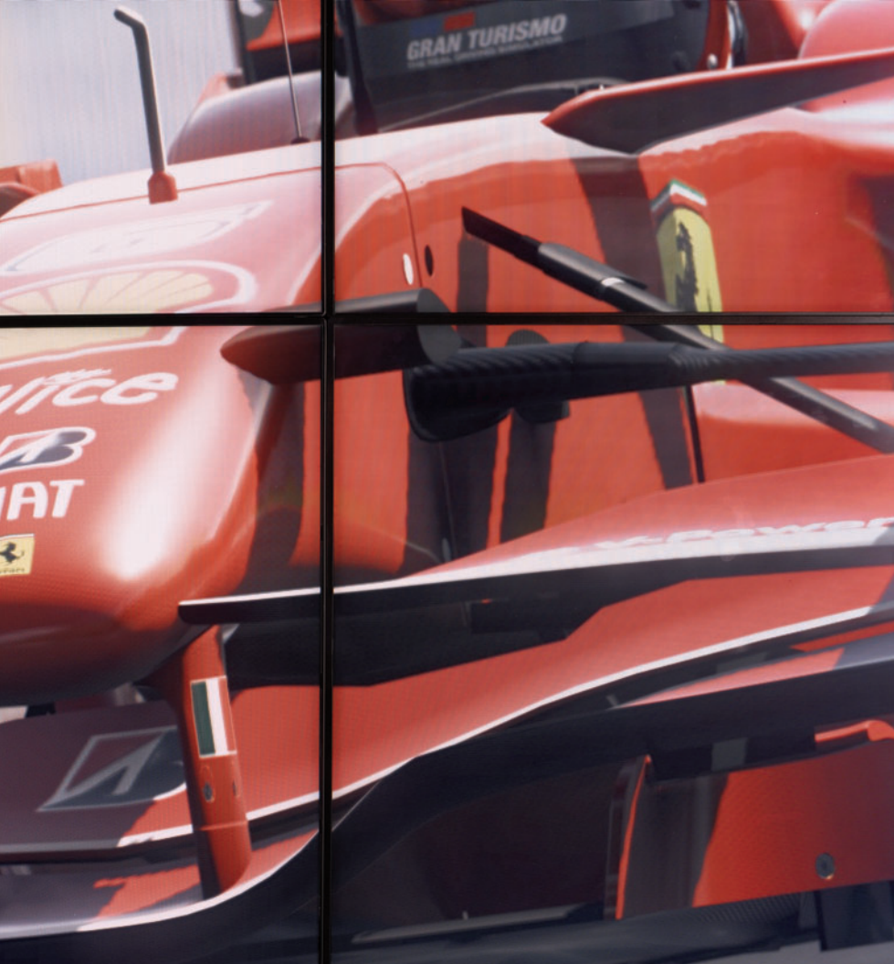
Seams between display panels are only a few millimeters
