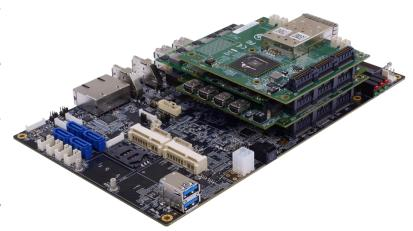
systems. This architecture evolved to address these resulting issues by keeping the common background while eliminating limitations. OXY5741 employs PCIe/104 technology to reduce constraints and create flexibility of expansion. Its M.2 extension offers M-key (M-Key 2280 optional), and PCIe 3.0 x 4 NVMe. Additionally, OXY5741 provides 3.0 ports for data redundancy by supporting RAID 0/1.
