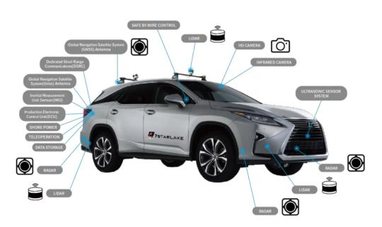
instrumented vehicle can consume over 30TB of data per day while a fleet of 10 vehicles can generate 78PB of raw data. Normally, the data rate of a camera is approximately 120MB/s while that of radar is close to 220 MB/s. To sum up, if a vehicle has a combination of 6 cameras and 6 radars, the complete vehicle
