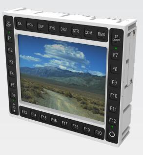
The GVD-126 GVA video display combines a rugged 10-inch touchscreen with real-time video imaging to provide a highperformance visualization display in a compact footprint. The GVD-126 display is compliant with the Generic Vehicular Architecture (GVA) and optimized for SWaP-C and modular open architecture, making this display ideal for vehicle-mounted C4ISR applications.
