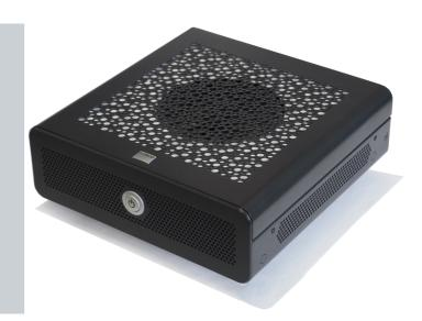
Barco's TransForm N NSD-110 is a compact and cost-effective video wall controller perfectly suited for visualizing networked video sources next to Windows local based applications. It enables customers to capture networked sources from anywhere and display them on a video wall up to 4 HD.
