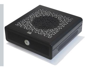
The EMS is part of Barco's innovative networked visualization solution. This device contains multiple services to process and redistribute up to 70 channels of streaming video. Compatible with a continuously growing list of encoders and cameras, the EMS combines versatility with best in class performance.
