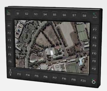
The SV-231 smart display from ScioTeq combines a 12-inch, high-bright touchscreen with the graphics and computing power of a rugged computer to provide a high-performance visualization processor in a compact footprint. With its design for SWaP-C and modular open architecture, this display is ideal for vehicle-mounted C4ISR applications.
