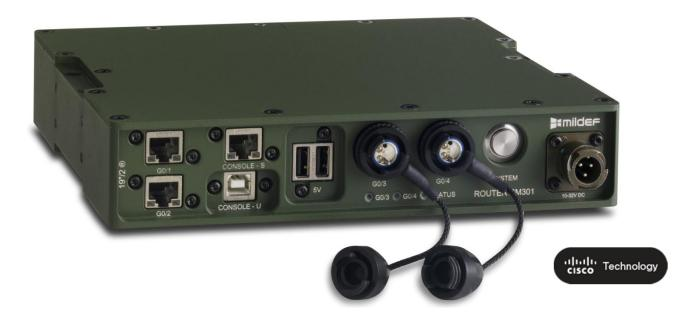
The 19"/2® Cisco Router RM301 is a high performance router in a compact and rugged design. It is based on the Cisco 5940 ESR card that features low power consumption and advanced network capabilities such as QoS. It supports Cisco IOS and is configured through the standard Cisco CLI.
