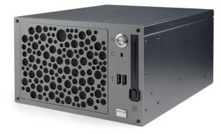
TransForm NSD-210 is a compact and cost-effective video wall controller perfectly suited for visualizing networked video sources next Windows local based applications. It enables customers to capture networked sources from anywhere, and display them combined in high resolution on a video wall up to 16 HD.
