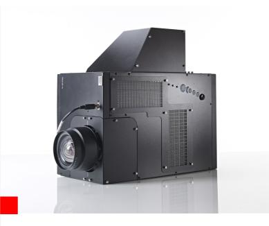
Powered by the latest generation of high contrast LCoS technology, Barco's SIM 7QP HC series was specifically designed for commercial flight, fast-jet and rotary-wing training systems. With a contrast ratio of up to 40,000:1, this is the projector of choice for demanding night and NVG training.
