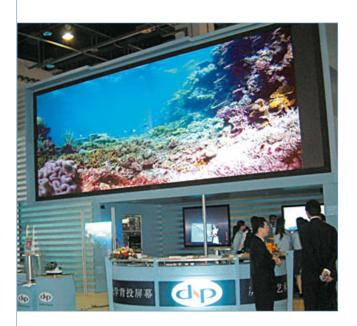
dnp Module Building System™ (MBS) is a seamless frame system for multi-screen applications in TV studios, video conferencing suites and small control rooms. The zero-seam frame system is designed for easy on-site assembly to reduce cost and hassle.
