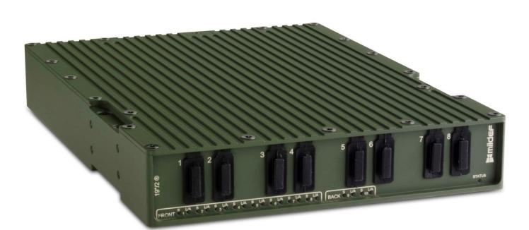
The  $19"/2^{\circ}$  10-p Fiber Switch ESW201 is a rugged Ethernet switch, which provides you with 10 SC fiber ports. There are three gigabit ports for single mode fiber and seven 100 megabit ports for multimode fiber. It is a high performance layer 2+ switch with a wide range of supported protocols.
