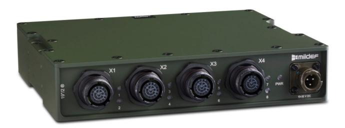
The 19"/2® 16-p Switch 8x2 ESW421 it's built from the inside and out for extreme environments. The 19"/2® form factor can save up to 75 % space compared to a standard 19" switch. It has aluminum casing and is made for operations down to -40 °C. The Ethernet ports also conforms to GVA Def Stan 23-09.
