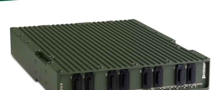
The 19"/2® 10-p Fiber Switch ESW202 is a rugged Ethernet switch, which provides you with 10 SC fiber ports and five rugged RJ45 connectors with PoE. There are three gigabit ports for single mode fiber and seven 100 megabit ports for multimode fiber. It is a high performance layer 2+ switch with a wide range of supported protocols.
