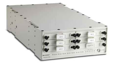
Storage computer in 19"/2 form factor The 19"/2 Storage Computer ST301 combines raid capability over several disks together with high speed output at 10Gb.
