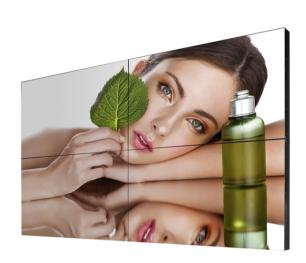
The OverView MVD-5521 is a 55" LCD panel with a super narrow bezel, making it ideally suited for tiled video walls. This LCD display uses IPS (In-Plane Switching) technology for consistent and accurate colors from all viewing angles, no blackening effects caused by light or heat, and stable response times. Unlike TN technology, IPS panels do not lighten or show tailing when being touched.
