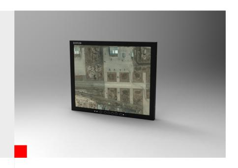
17" semi-rugged touch display with SXGA resolution for naval and shelter applications.
