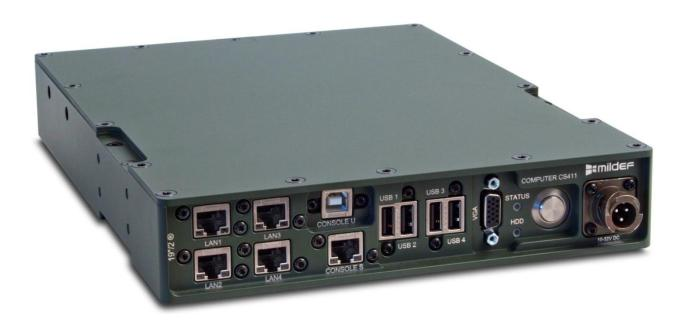
The 19"/2 Computer Atom CS411 is a rugged computer with the processing power of an Intel Atom D2550 1.86GHz processor in a compact, small 19"/2 form factor. The CS411 is optimized for size, weight and power consideration, with low power consumption and a weight of 3 kg. Designed for rugged military applications in tough environments.
