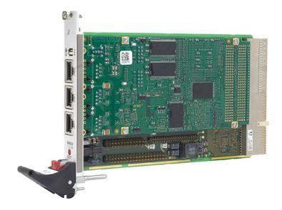
the MPC5200B and are accessible via SA-Adapters. A second serial interface can be accessed using an SA-Adapter on the F12N. (E)IDE and GPIO are also on board.
