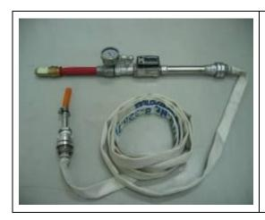
Internal diameter of the nozzle : 6.33mm
