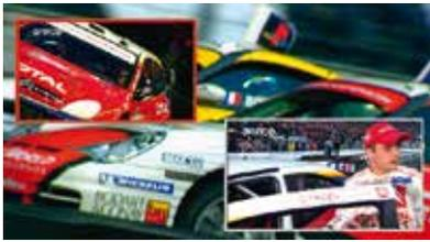
The 2D-DVE card allows you to create PIPs from any source. A wide variety of effects are offered, including sizing, positioning, cropping, and programmable borders and shadows.
