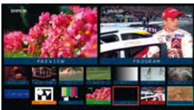
The Multiviewer card provides a fully integrated monitoring solution, eliminating the need for multiple monitors and signal distribution, simplifying your system's operation and reducing the overall operating cost. The Multiviewer enables you to monitor up to 16 video signals, comprised of any input source, any Program, Preview or Clean feed output, and any Aux bus output.
