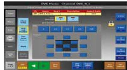
The system’s DVE menu provides an easy and intuitive way to set up and run each DVE channel. All buttons are color-coded according to functionality, and on the menu’s “size and position” tab, the central palette contains dedicated presets for rapid and accurate effect creation. Additional tabs are provided for effect setup, panning and zooming the source within a PIP, masking all edges, and creating borders and shadows.
