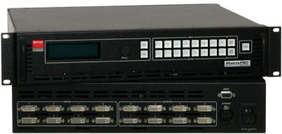
The MatrixPRO 8x8 DVI router accepts inputs up to 2048 x 1080 (including all HD) resolutions. Each input is re-clocked as it passes through the router maintaining the DVI signal strength. Each output channel can also display an internally generated test pattern. The test patterns are available with or without any valid input signals.
