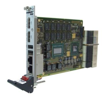
The board delivers an excellent graphics performance. Two DisplayPort<sup>®</sup> interfaces are accessible at the board front. Using an external adapter two HDMI or two DVI ports can also be realized. In addition the standard front I/O comprises two PCIe<sup>®</sup>-driven Gigabit Ethernet and two USB 2.0 ports.
