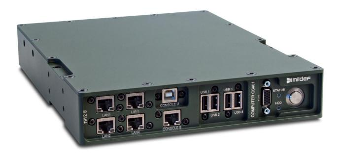
The 19"/2 Computer Atom CS401 is a rugged computer with the processing power of an Intel Atom D2550 1.86GHz processor in a compact, small 19"/2 form factor. The CS401 is optimized for size, weight and power consideration, with low power consumption and a weight of 3 kg. Designed for rugged military applications in tough environments.
