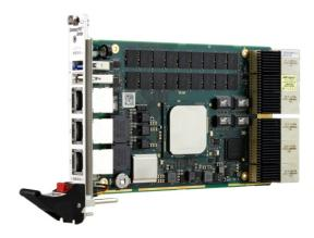
The memory configuration of the G25A includes a stateof-the-art fast DDR4 DRAM with ECC which is soldered to the board to guarantee optimum shock and vibration resistance. A microSD card device which is connected via a USB interface offers space for user applications or as a local boot medium.
