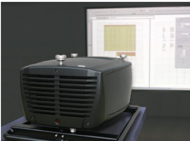
*The SXGA+ resolution (1400 x 1050 pixels) of the CLM R10+ offers 87% more pixels than the XGA panels used in high brightness LCD projectors.*
